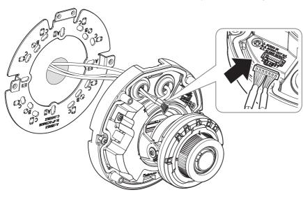
9. Join the camera body with the mount plate.
