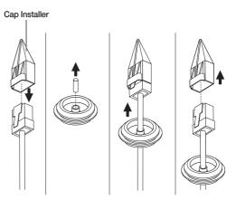
4. Insert the cable bushing of the network cable into the camera body.
