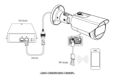
The Micro USB port of the product is provided for easier installation, and is not recommended for monitoring purposes.
