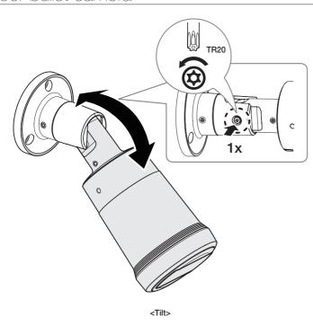
When adjusting the camera monitoring direction, loosen the corresponding fixing screws, adjust the camera, and then tighten
