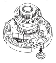
7. Insert the cable bushing of the audio/alarm cables into the camera body.
