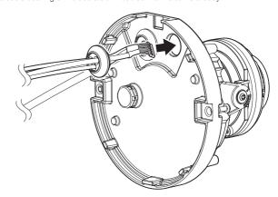
8. Connect the audio/alarm cable connector to the audio/alarm cable port of the camera body.
