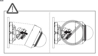
Adjust the direction of IR LEDs not to hinder their view by an instrument.
