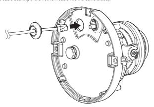
5. Connect the network cable connector to the PoE port of the camera body.
