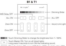
When the light is ON, press "60S Delay OFF", the light will be OFF Automatically after 60 seconds.
