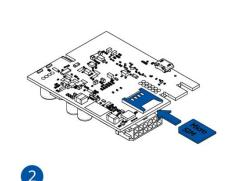
Figure 5 Micro-SIM card insert
