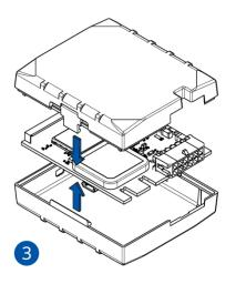
Figure 6 Attaching cover back
