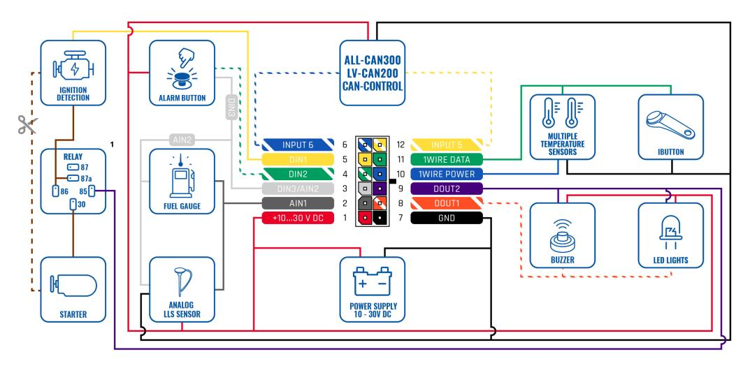
Figure 3 FMB110 Wiring scheme
