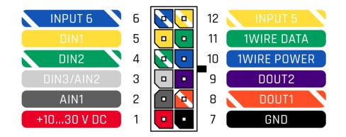
Figure 2 FMB110 2x6 socket pinout
