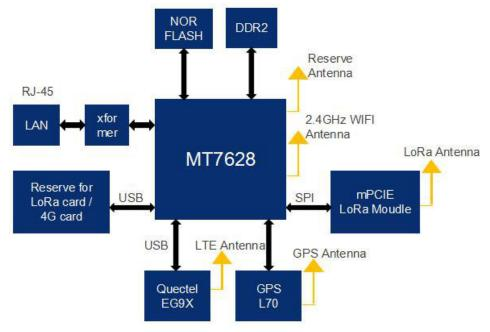
Figure 4 | Block Diagram
