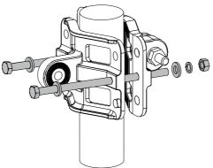
**Step 3:** Connect the clamp and the bracket on the backside of the casing with hexagonal bolts M6x30, washers and nuts
