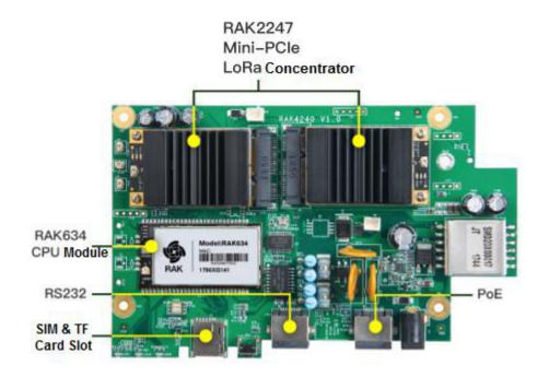
Figure 5 | Circuit Board
