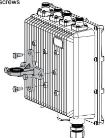
**Step 2:** Tighten the pole clamp with hexagonal bolts M6x110, washers and nuts
