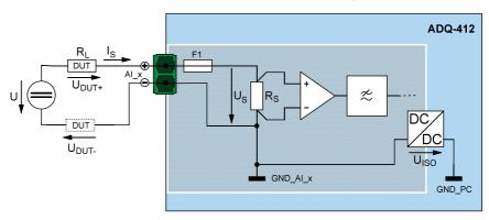
Figure 5: Wiring the current measurement channels
