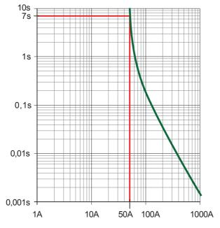
Figure 8: Characteristic of the fuse
