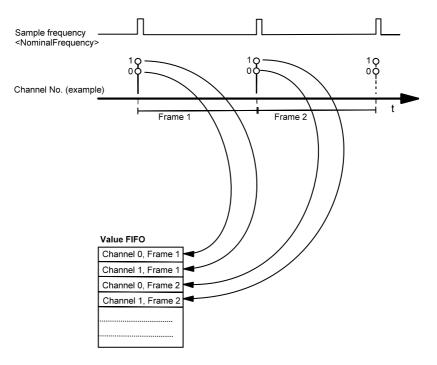
Figure 7: Timer-controlled acquisition
