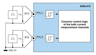
Figure 6: Wiring of the external trigger inputs
