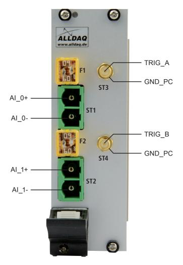
Figure 9: Connectors of the ADQ-412
