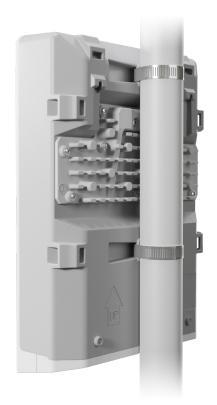
netPower 16P has a non-blocking throughput of 36 Gbps, switching capacity of 72 Gbps and forwarding rate of 53.6 Mpps.
