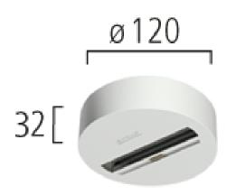
Synergy 21 by EUTRAC 3~UPPOINT OUTLET WITH BUS, white with data bus contact suitable for 3-phase MultiAdapter and UniCompactAdapter with and without data bus tap and universal adapters from other manufacturers, max. length 95 mm, loadable up to 10 kg
