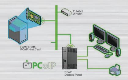
The TERA2140 PCoIP workstation client ships with four 1Gbit of DDR3 memory and supports four DVI, four USB, a Speaker, a Microphone, a Headphone and an Ethernet connectors (with RJ45 or SFP Fiber connector). Output is driven by the DVI ports for video and USB 2.0 ports for peripheral and I/O connections. The net result is a fan-less and reliable client-side device that requires minimal IT administration and support since all processing resides on the host PC or workstation.
