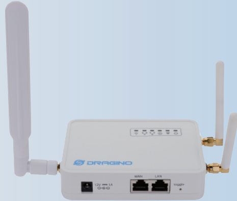
Dual Channel LoRa Gateway Indoor & Outdoor version
