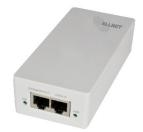
With the ALLNET ALL0488V5 Power over Ethernet Injector you can install your Ethernet-enabled IP devices such as wireless access points, VoIP phones and much more totally independent of existing electrical outlets.
