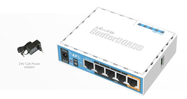
The hAP ac lite can be powered from the power jack or with passive PoE from a PoE injector. The power adapter is included. Unit provides PoE output function for port 5 - it can power other PoE capable devices with the same voltage as applied to the unit. Maximum load on the port is 500mA.
