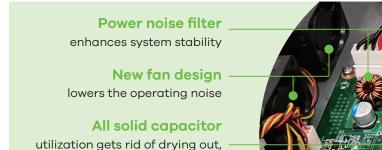
bursting and leaking problems
