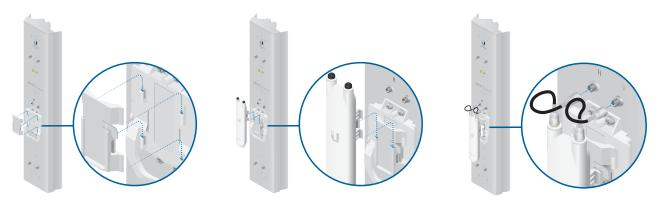
The included fast-mount adapter attaches to the radio mount of an optional airMAX antenna.
