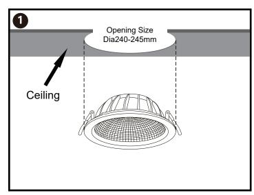
Prepare everything needed for installtion & drill a hole with diameter 240-245mm in the ceiling.
