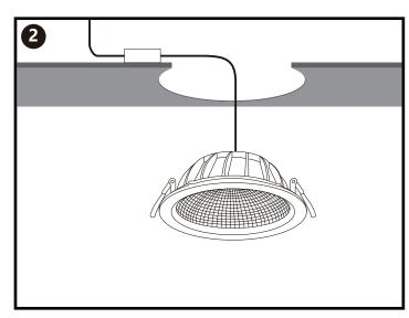
Connect the input side to the LED driver.
