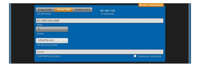
**SSID:** You can enter any network name here. This name is displayed when the network is scanned.
