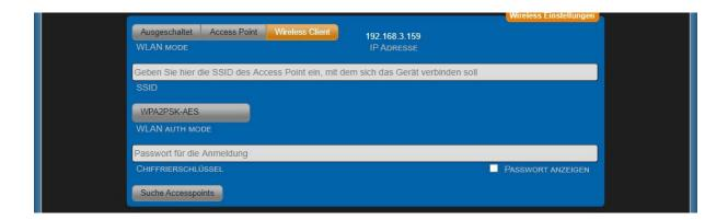
Select Wireless Client to connect the device to an existing network. Click on "Search access points" to search for your WLAN network.
