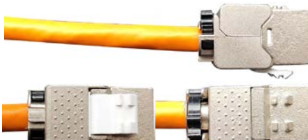
⑩.Fasten smart cable ties for 360 degree shielding
