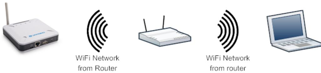
If the LPS8 already connect to the router via WiFi, use can use the WiFi IP to connect to LPS8.
