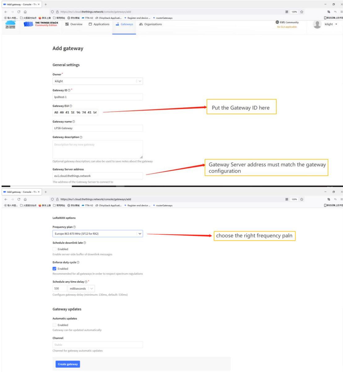
**Notice:** Gateway Server address must match the gateway configuration, otherwise you will have problem for End Node to join the network.
