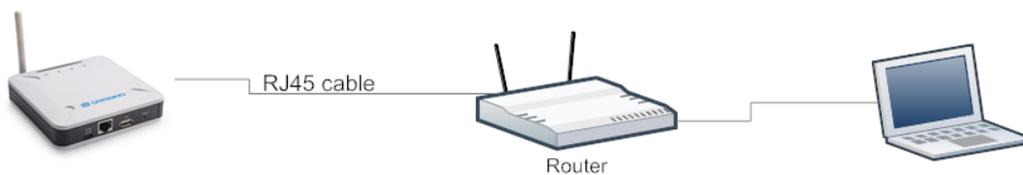
Alternatively, connect the LPS8 Ethernet port to your router and LPS8 can obtain an IP address from your router. In the router's management portal, you should be able to find what IP address the router has assigned to the LPS8. You can also use this IP to connect.
