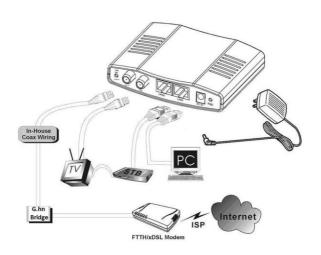
The figure above shows how to connect an xDSL modem to a home coaxial cable network. Follow the same steps to connect any Ethernet device such as a HUB or printer, to a coaxial cable network.
