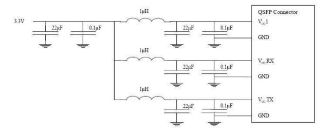
Figure 1. Host Board Power Supply Filtering
