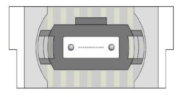
Transmit Channels: 1 2 3 4 Unused positions: x x x x Receive Channels: 4 3 2 1
