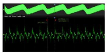
Utilizing a hardware-based Zoom technique and record length up to 200 Mpts, users can select a slower timebase without compromising the sample rate and then quickly zoom in to focus on the area of interest.
