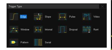
Edge, Slope, Pulse, Video, Windows, Runt, Interval, Dropout, Pattern and serial trigger.
