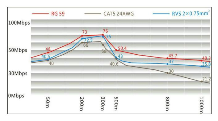
The above data are parameters of a one-way network. The tests were carried out under the condition that the cable is not completely removed. There may be differences compared to the practical application of the data. The rate is only used as a reference for the project application.
