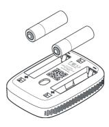
Replace the batteries with two new AA type batteries. Pay attention to the polarity.
