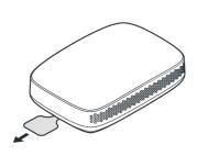
Pull the battery tab to activate the sensor
