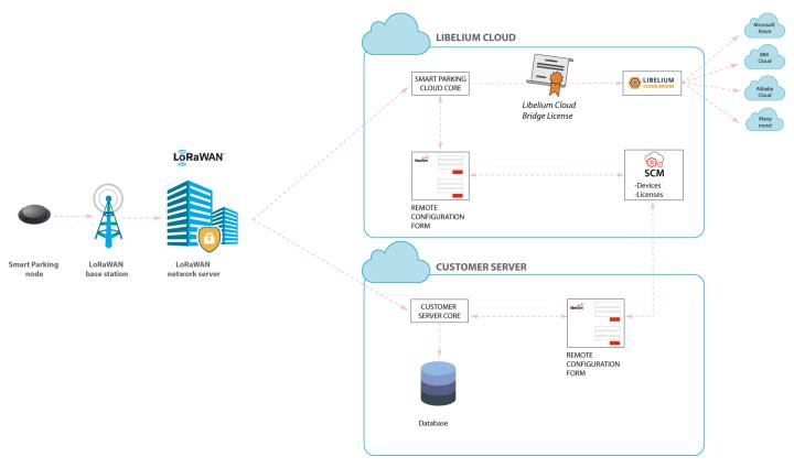
Figure : Smart Parking network architecture
