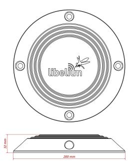
Figure : Flat Smart Parking enclosure dimensions
