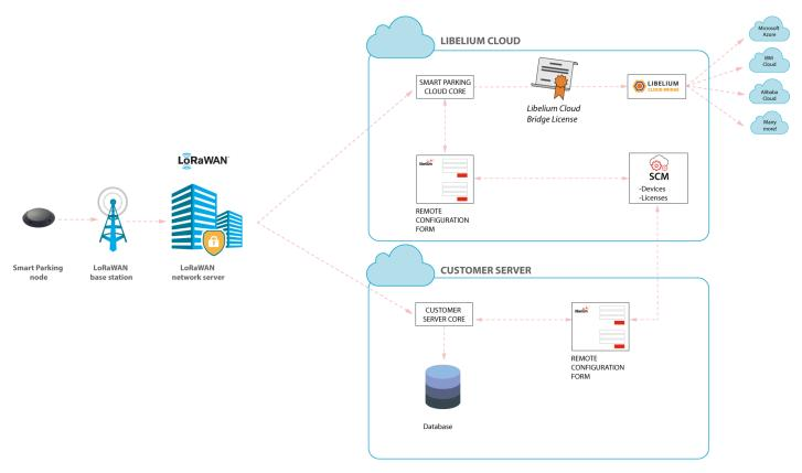
*Figure : Smart Parking network architecture*
