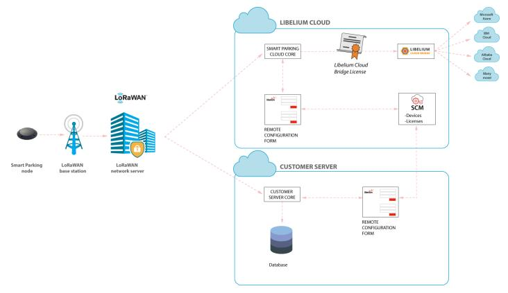
Figure : Smart Parking network architecture
