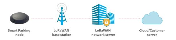
Figure : Simplified Smart Parking network architecture
