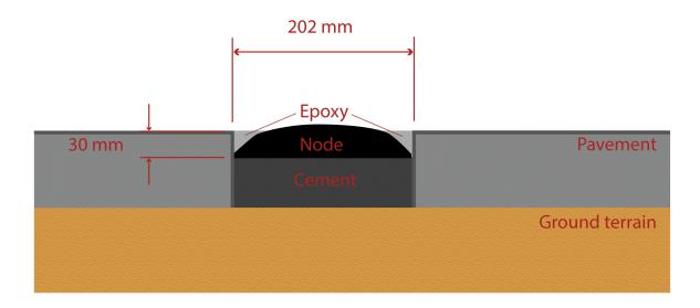
Figure : Semi-underground node installation
