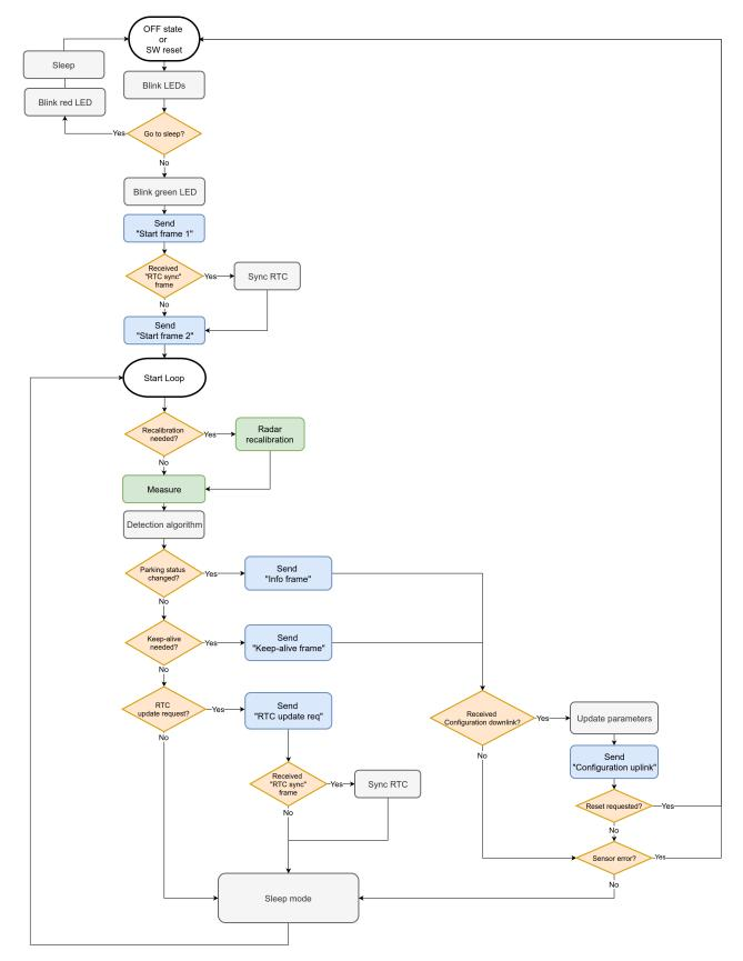
Figure : Smart Parking node program flowchart
