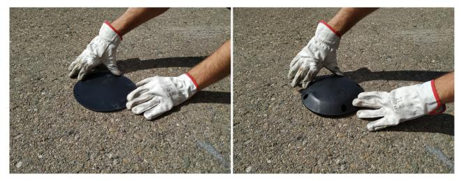
Figure : Place the circle rubber and the node above it
