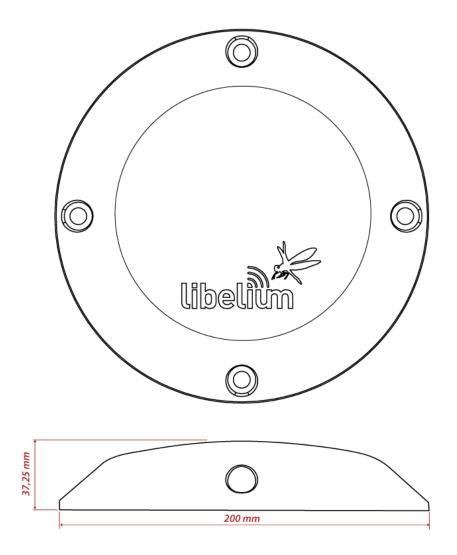
Figure : Vaulted enclosure dimensions
