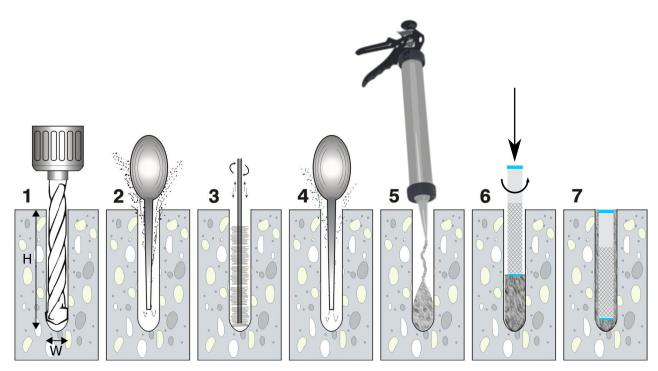
*Figure : Step by step chemical fixing and anchor installation*
