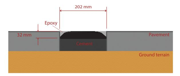
*Figure : Placing the node in the hole*
