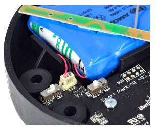
Figure : Smart Parking node "user switches"
