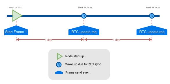
Figure : Example of RTC sync
