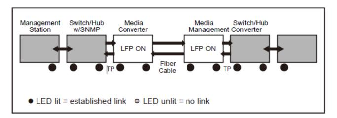
If the connection breaks, RM202-1GF1GT that link loss forward to the Switch / Hub that generates a trap to the management station. The administrator can then determine the source of the problem.
