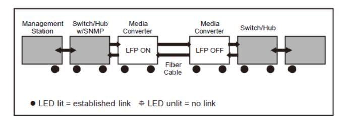
If one of the optical conductors is down (as shown in the diagram box below), the converter with LLR function will return a no-link condition to its link partner. With LLCF function also enabled, the no-link condition is carried forward to the switch/ hub where a trap is generated to the management station, and the administrator can then determine the source of the loss.
